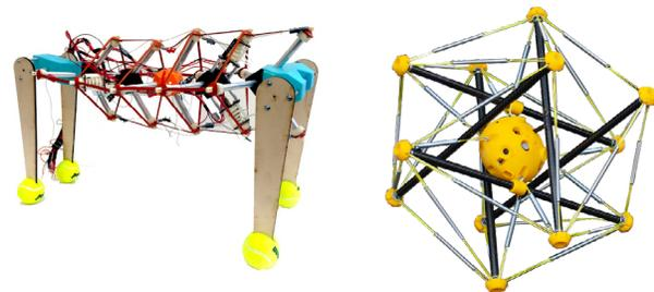
Laika the quadruped robot with a tensegrity spine, Squishy Robotics a spin-off of BEST Lab research on tensegrity robots for space exploration. All images are courtesy of UCB BEST Lab.
