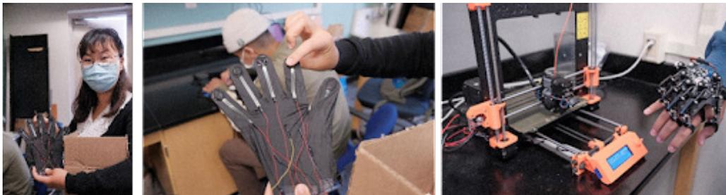
In tactile sensing and haptic control, we design, model and fabricate soft exoskeletons and wearable electronics. Among them is a wearable master-slave glove, which can communicate with haptic feedback wirelessly through ESP32. We are interested in using them for manipulation, teleoperation, and remote surgical training tasks.
