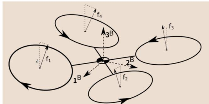
UAV with tilted propellers away from common thrust direction which helps improve total power consumption.
